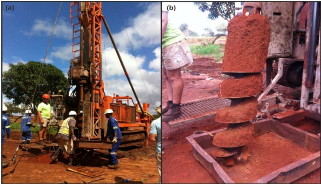
Figure 3-6: Auger drilling at Mugloto observed during the March 2015 site visit using a specially modified Sandvik DE700 diamond rig (a) with an auger drill bit (b)
