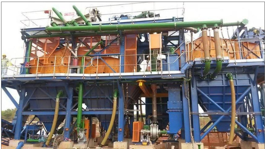
Figure 7-4: DMS plant showing feed screen, media pumping circuits, dense media cyclones and drain and rinse screen
