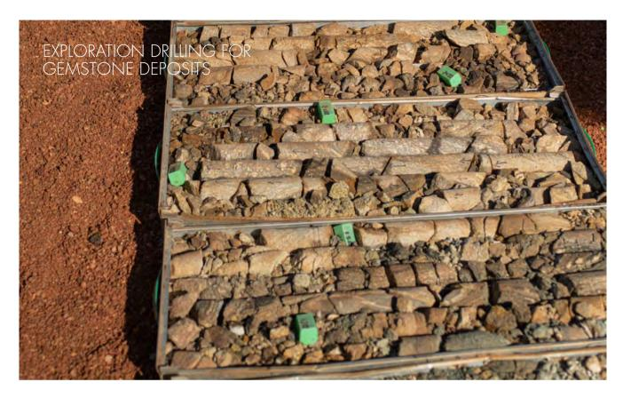
An exploration auger drilling campaign was initiated and a total of 2,500 metres from 616 boreholes was drilled on a 200 x 100 metre grid interval in a diamond pattern covering three sub-blocks. The secondary ore samples intersected during the auger drilling were processed in two Bushman jigs. Six boreholes recovered ruby and tumble incidences with 0.010 and 0.14 g whereas three boreholes recovered sapphire with 0.14 g.
