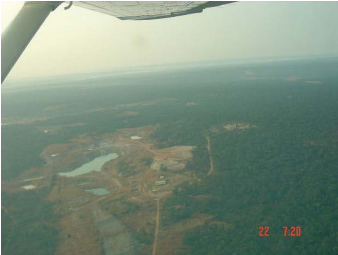
PHOTO 1. AERIAL PHOTO OF LARGER KAMAKANGA PIT AND SMALLER JAI AMBE PIT BEYOND WASTE DUMP IN LEFT FOREGROUND, WASHING PLANT TO THE RIGHT OF JAI AMBE PIT AND WORKSHOP IN RIGHT CENTRE
